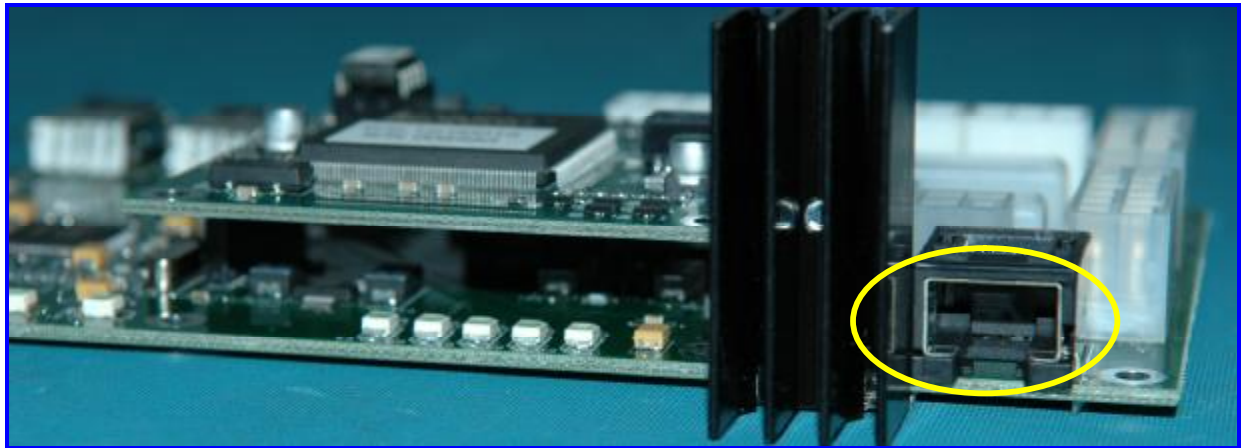
Rear view of the BMIX002A circuit board, showing the RJ-45 connector at the right.
